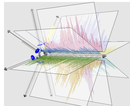
**Figure 2** A 3D Multi comb representing eight time-dependent attributes as plots with respect to a common central time axis.
